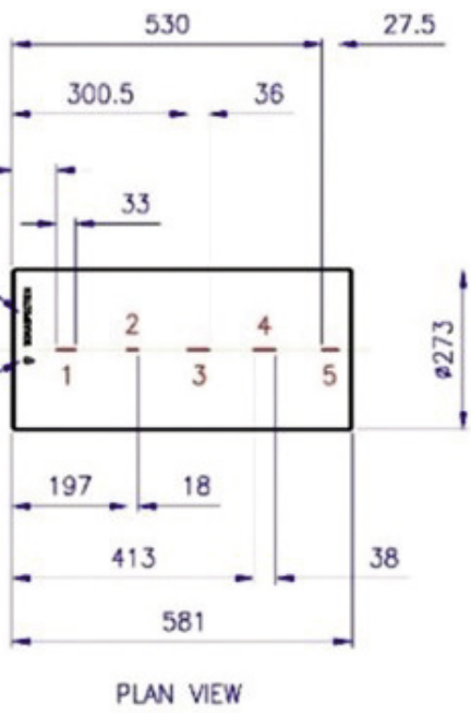
ToFD drawing overview of ERW seam
