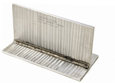
An example of a magnetic testing tee specimen
