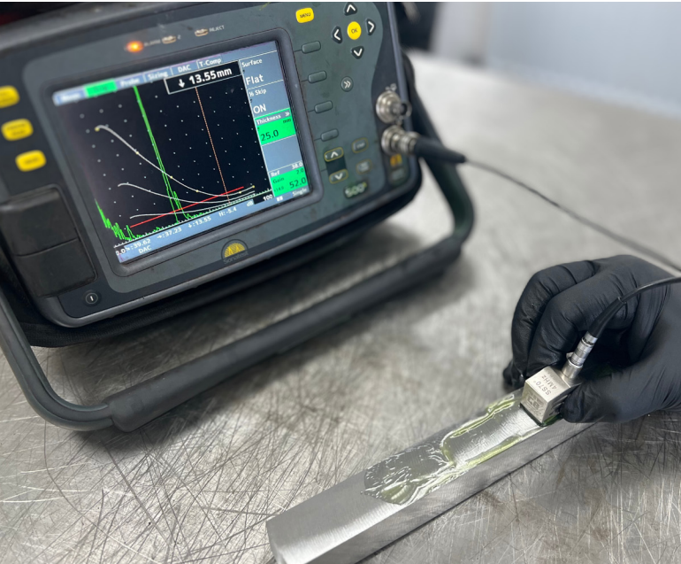
An example of a crack sizing bar
