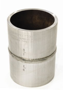
An example of a penetrant testing pipe specimen
